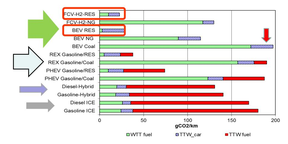
CO<sub>2</sub> emissions per km driven for various types of EV in comparison to conventional cars (power of car: 80kW)
