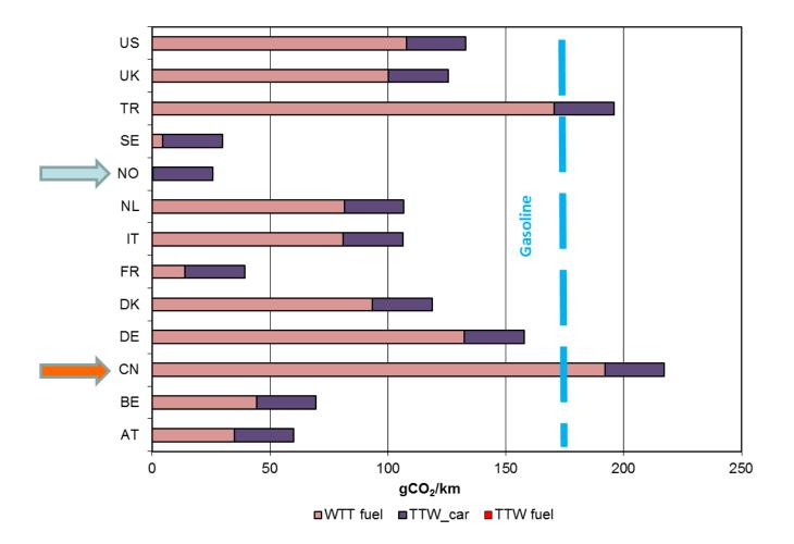
CO<sub>2</sub> emissions per km driven for BEVs powered by grid electricity in different countries
